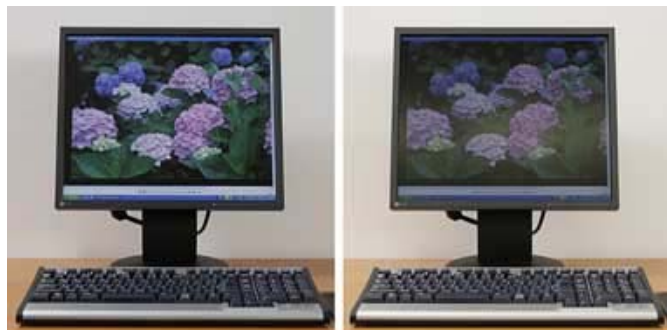
Fig.2: Image on Non-Glare LCD (The photo was taken under the same condition as Fig.1.)
