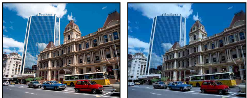
Compared to a color temperature of 5000K (L), the same image is noticeably bluer at 9300K (R).
