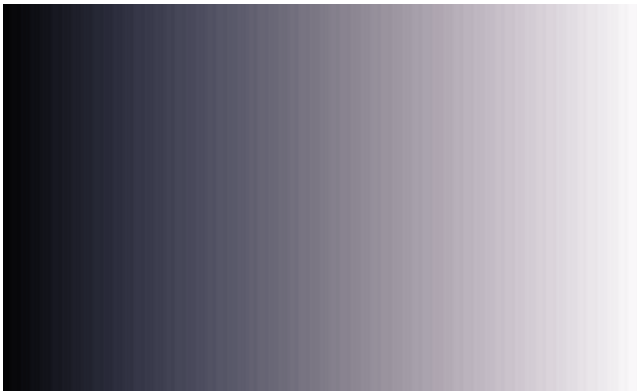
With software calibration, color seepage and banding are visible in a grayscale ramp.
